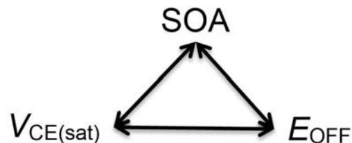
Figure 2: Fundamental trade-off for IGBT characteristics
