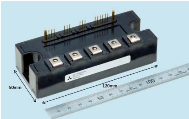
Figure 1: S1-series package outline, Baseplate footprint: 50x120mm
