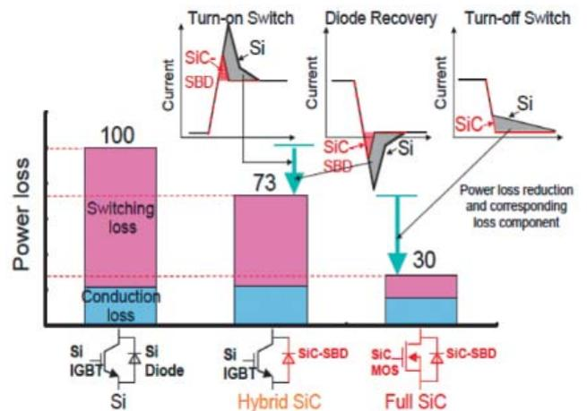
Figure 2: Evolution of SiC technology in power modules
